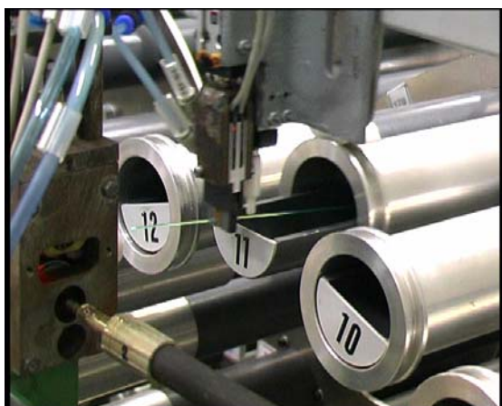
Figure 15: Cartesian robot picking a fibre
