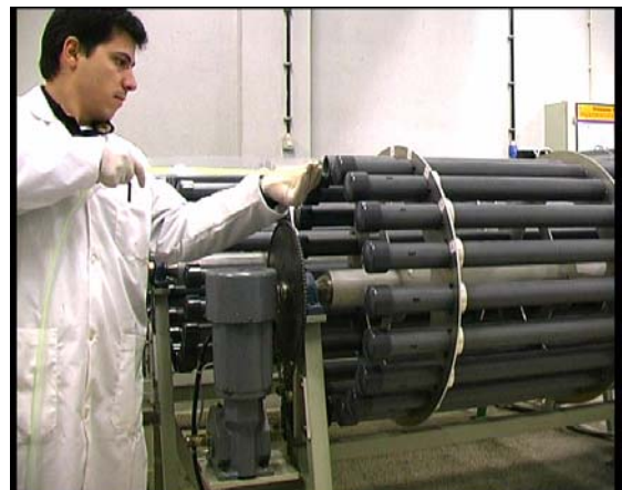
Figure 13: Operator inserting fibres inside the drum
