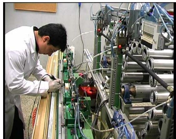
Figure 22: Operator doing the gluing operation
