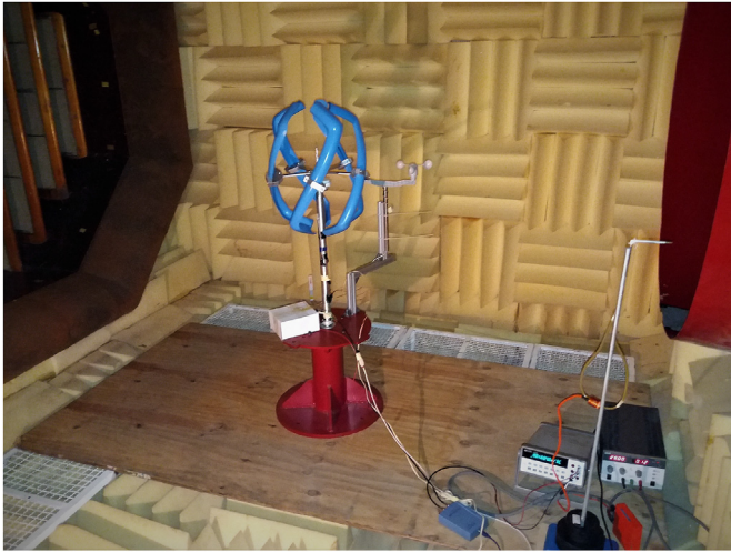
Fig. 15. Aeroacoustic wind tunnel Setup. Prototype and pitot tube installation.
