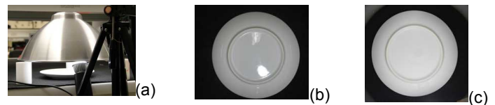
Fig. 2. (a) Dome used to take pictures and images without (b) and with dome light (c)
