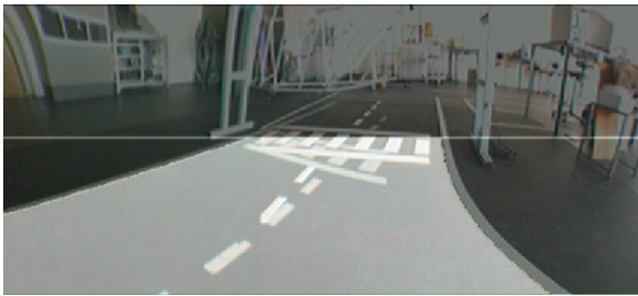
Figure 5 - The original merged image. The segmented road area is overlaid in white.
