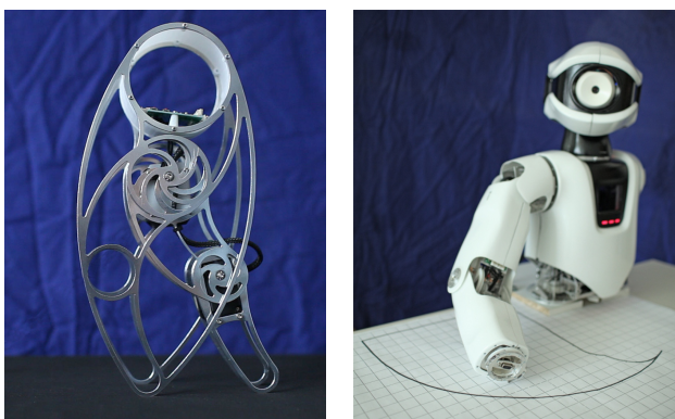
Figure 2. Left: The 30 cm tall robot SEMNI standing in an upright position. Proprioceptive sensors are located within the actuators (hip, knee) and on the printed circuit board in the head. The robot is facing to the left, with the leg standing on the back side. Right: Head, torso, and right arm of the modular humanoid research robot Myon. The black solid line indicates the area which can be reached by the arm. The hand is not attached in this experiment.
