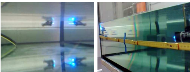
Fig. 6. (Left) Autonomously swimming AUV recognizes obstacles with the digital S&C system (active sensing); (Right) Experiments with digital communication.
