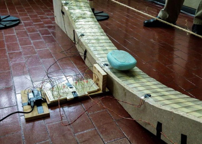
Fig. 5. Photo of the rail with the optical sensors distributed along the track, and the Arduino microcontroller circuit to process all sensors data.
